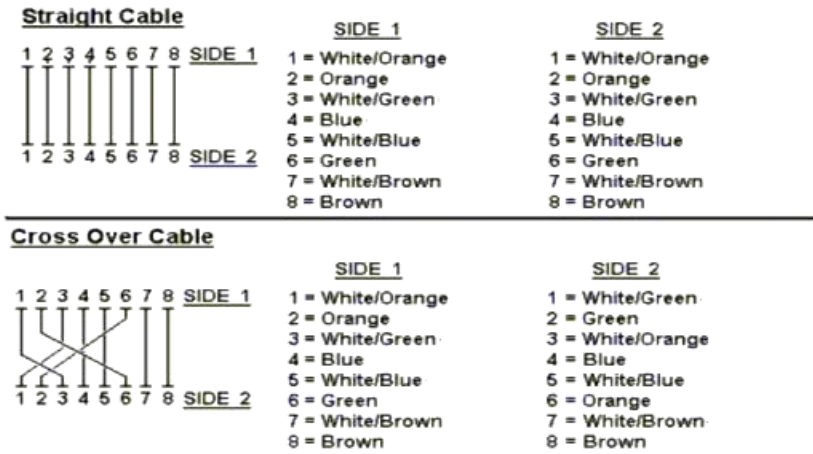
Figure A-1: Straight-Through and Crossover Cable
